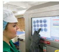
Figure 7 Maximum permitted leakage levels from an x-ray system: 1 mSv/year (RoW regulations), 5 mSv/year (US regulations)
